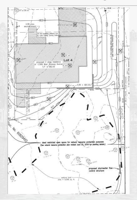
Staff has worked with applicant to design a stormwater capture system that redirects and improves current drainage in the vicinity of the property
