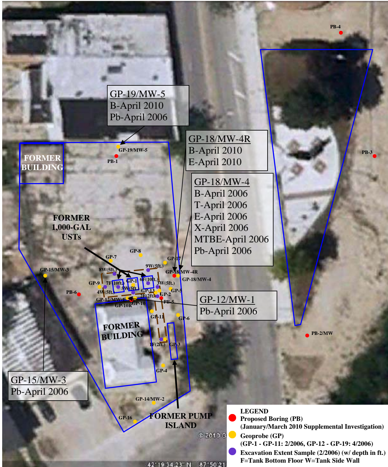
Figure 5 Groundwater Concentrations Exceeding Class I Groundwater Objectives 1820 Sheridan Rd. North Chicago, IL 60064
