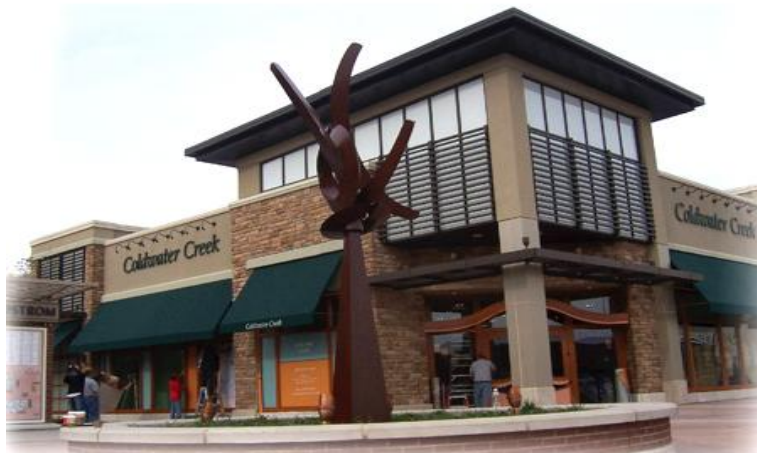
Encouraged: Use of roof structure to hide mechanical equipment.
