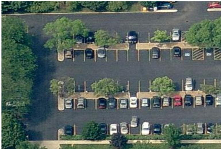
Encouraged: combination of open curbing, bio-filter and plantings to treat stormwater.
