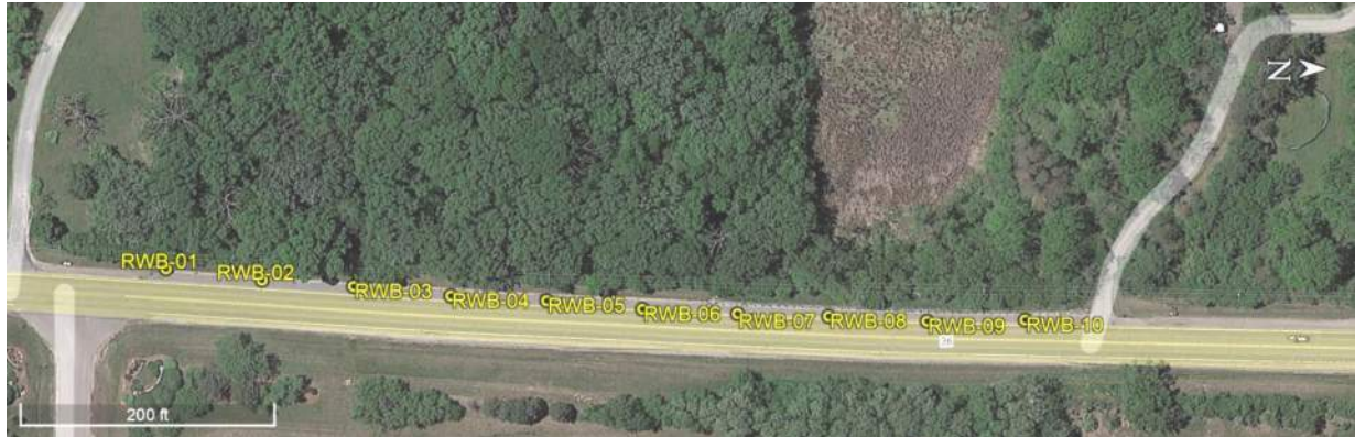
Exhibit 1) Proposed boring locations in SB shoulder of Deep Lake Road for south wall
