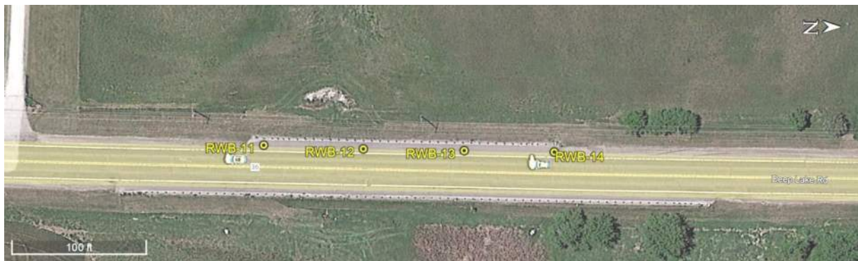
Exhibit 2) Proposed boring locations in SB shoulder of Deep Lake Road for north wall
