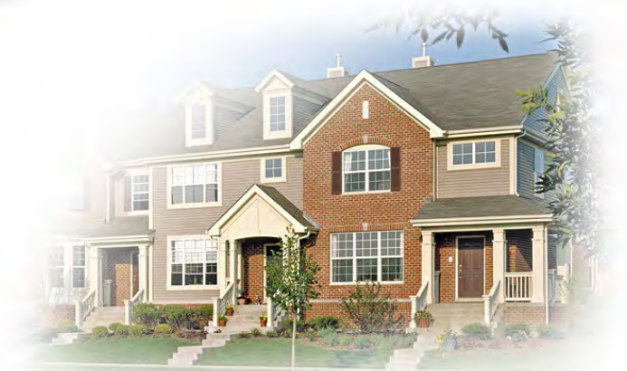
Examples of acceptable Attached Single-Family facade designs indicating the use of elements such as dormers, bay window projections and dominant entry features.
