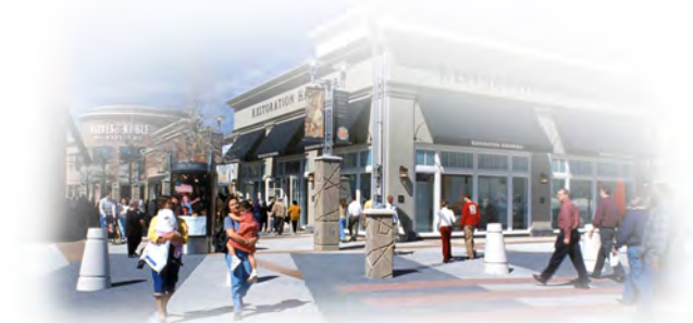
Example of protective bollards in pedestrian walkway
