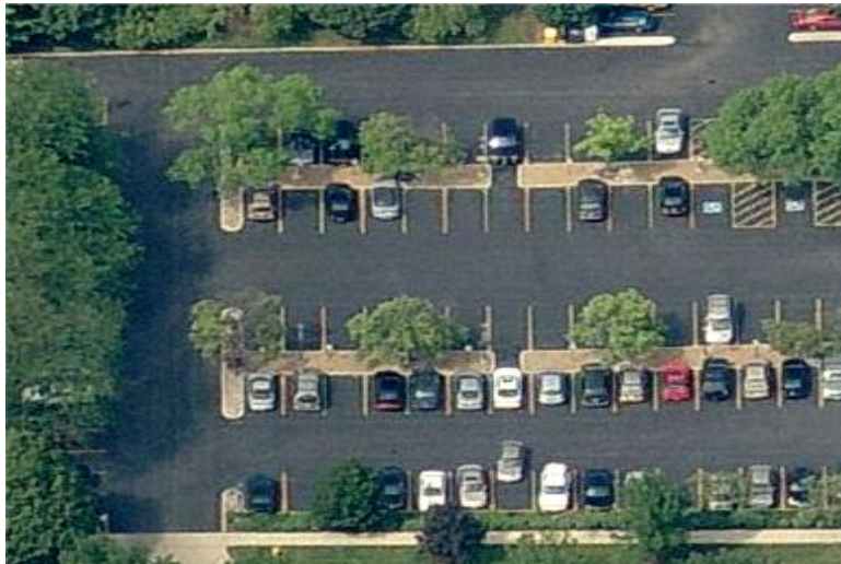
Encouraged: combination of open curbing, bioswale and plantings to treat stormwater.
