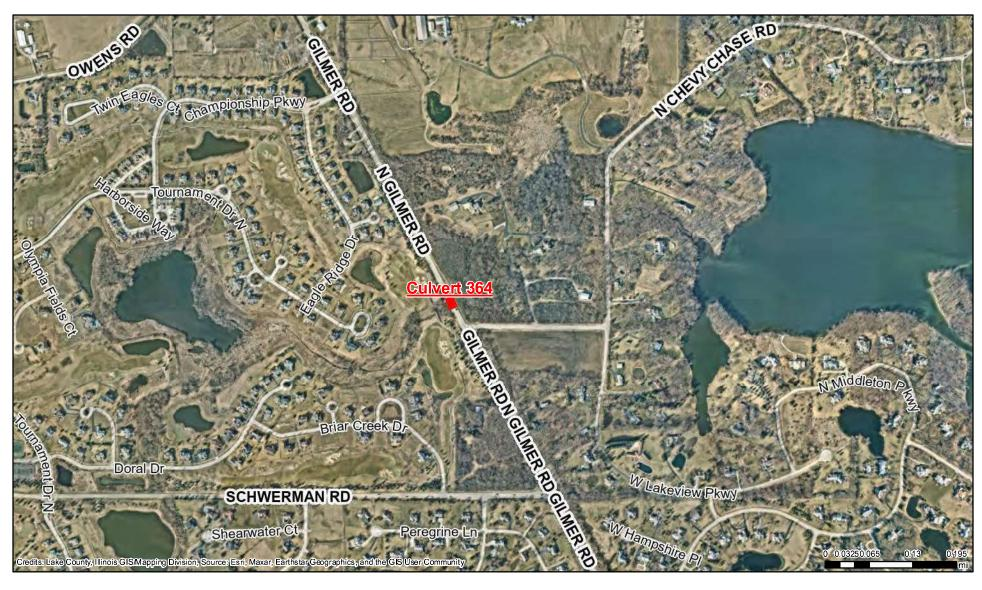
Culvert 364 - Gilmer Road (North of Chevy Chase Road) 30" Concrete Pipe - Installed 1993 Flared End Section to No End Section Unable to rate due to both end sections being under water (2022) \*Consider Upsizing and Raising Culvert \*Verify Culvert is Within R.O.W.
